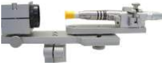
7-2 Install the fiber connector under microscope
