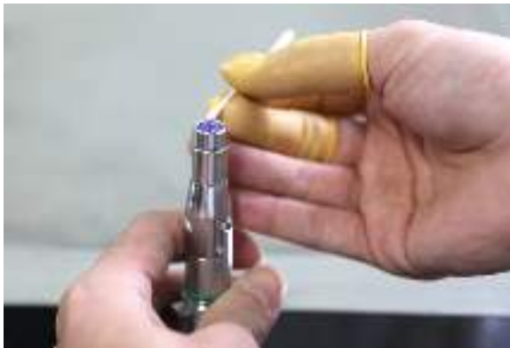
7-3 Cleaning protective lens with swabs
