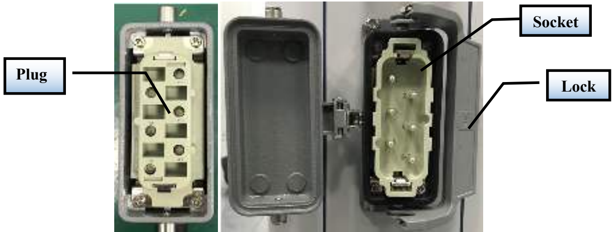
a) The picture of 3.3kW / 4kW power port plug / socket.
