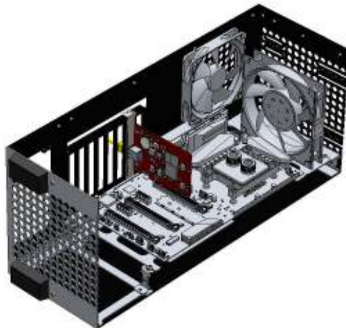
Figure 5 BMC228A Control Card After Installation
